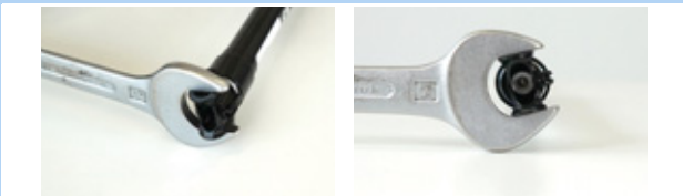
Figure 190: Securing against twisting
