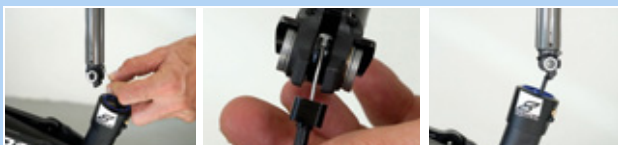
Figure 227: Attaching and pushing in the seat post
