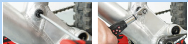
Figure 199: Fastening the Postpin axle
