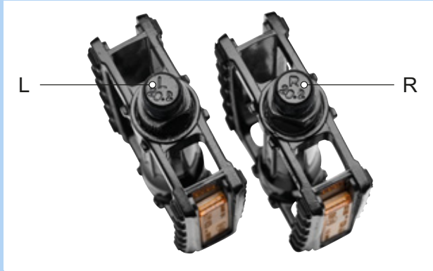
Figure 67: Example of markings on pedals
