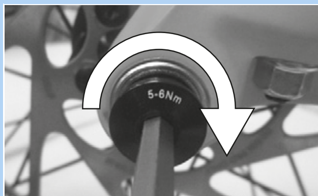
Figure 56: Tightening the securing screw
