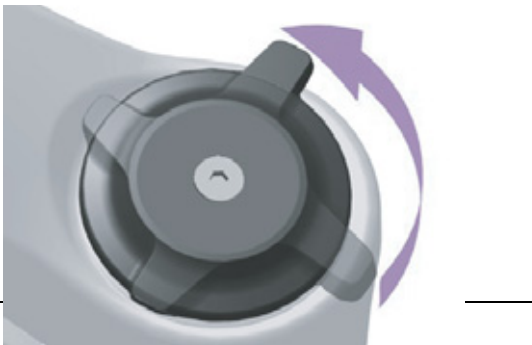
Figure 148: Changing compression adjuster to a softer setting
