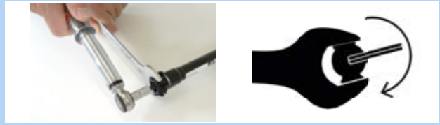
Figure 191: Setting in a clockwise direction
