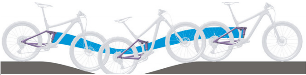
Figure 259: Excessively soft suspension in the rear frame damper on hilly terrain
