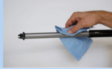
Figure 222: Cleaning the longitudinal groove
