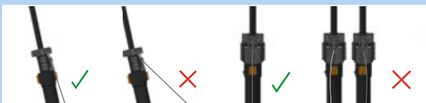
Figure 196: Correct and incorrect Bowden cable
