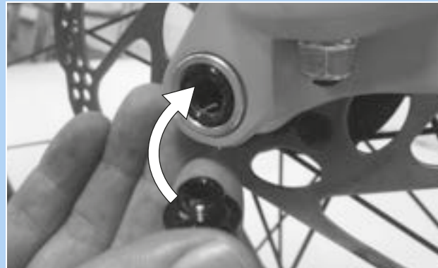
Figure 55: Pushing the quick release lever into the axle
