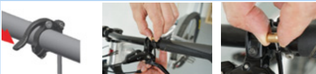
Figure 171: Removing the cartridge
