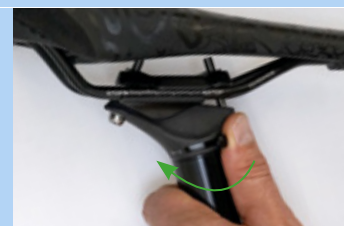
Figure 225: Closing the height adjustment
