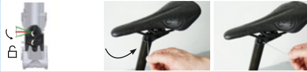
Figure 169: Moving height adjustment to the “Open position”
