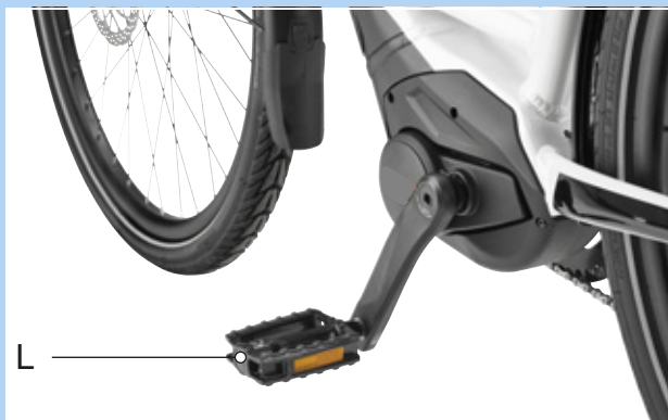
Figure 68: L-pedal in the left-hand crank arm
