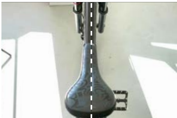
Figure 71: Positioning the saddle in direction of travel
