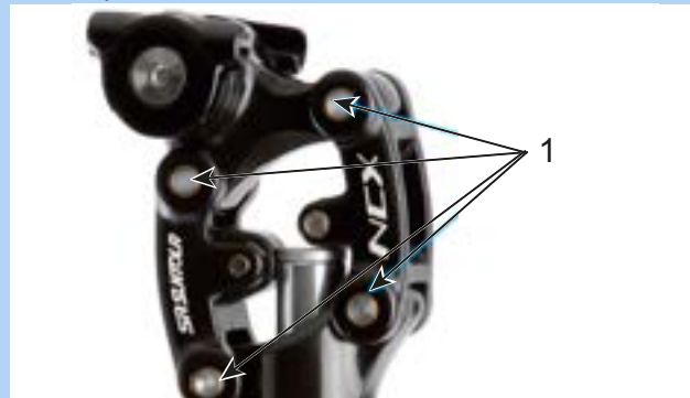
Figure 168: SR Suntour suspension seat post lubrication points
