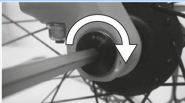
Figure 54: Tighten the axle in the direction of the arrow
