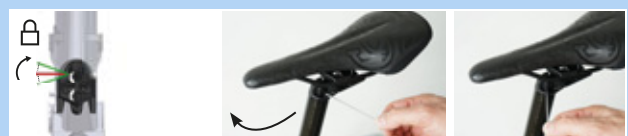
Figure 206: Closing the height adjustment
