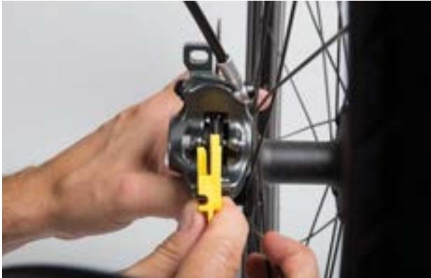
Figure 158: Checking the brake lining when fitted with the help of the transport safety wear gauge
