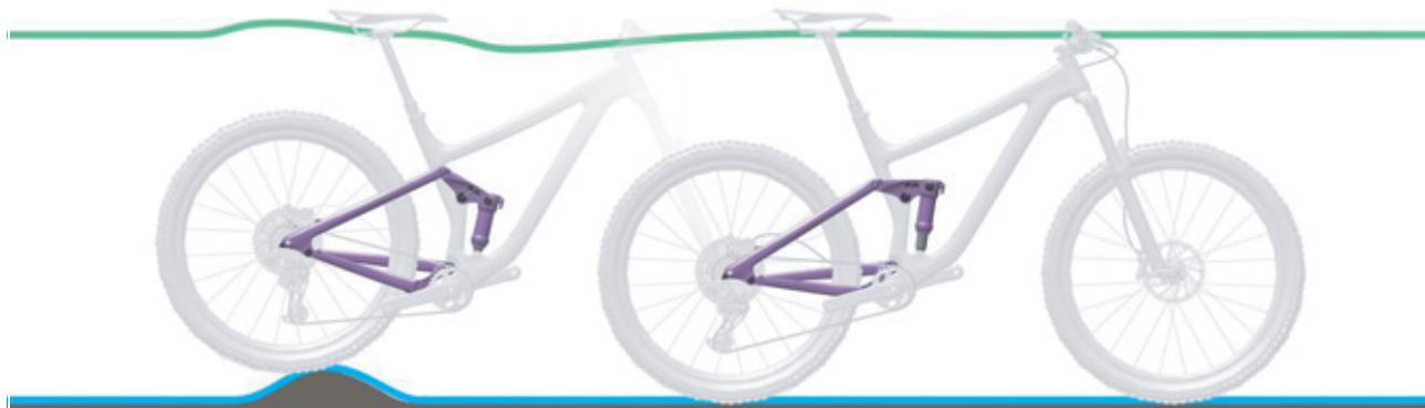
Figure 119: Optimum rear frame damper ride performance over bumps
