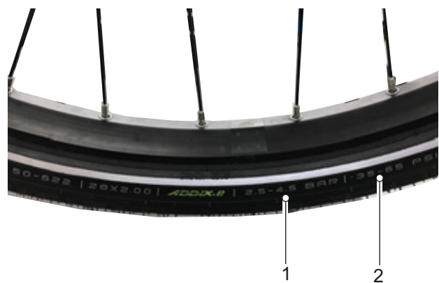
Figure 155: Tyre pressure in bar (1) and psi (2)
