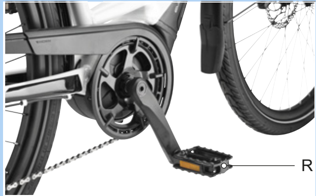
Figure 69: R-pedal in the right-hand crank arm
