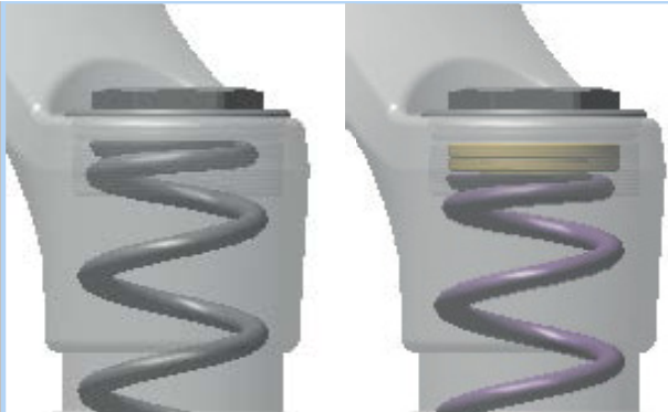
Figure 111: Screwing and unscrewing the preload adjustment ring
