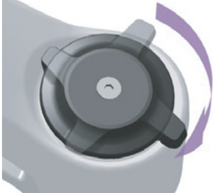
Figure 147: Changing compression adjuster to a harder setting
