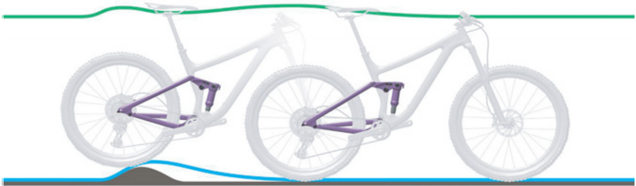
Figure 253: Excessively hard damping in the rear frame damper on bumps
